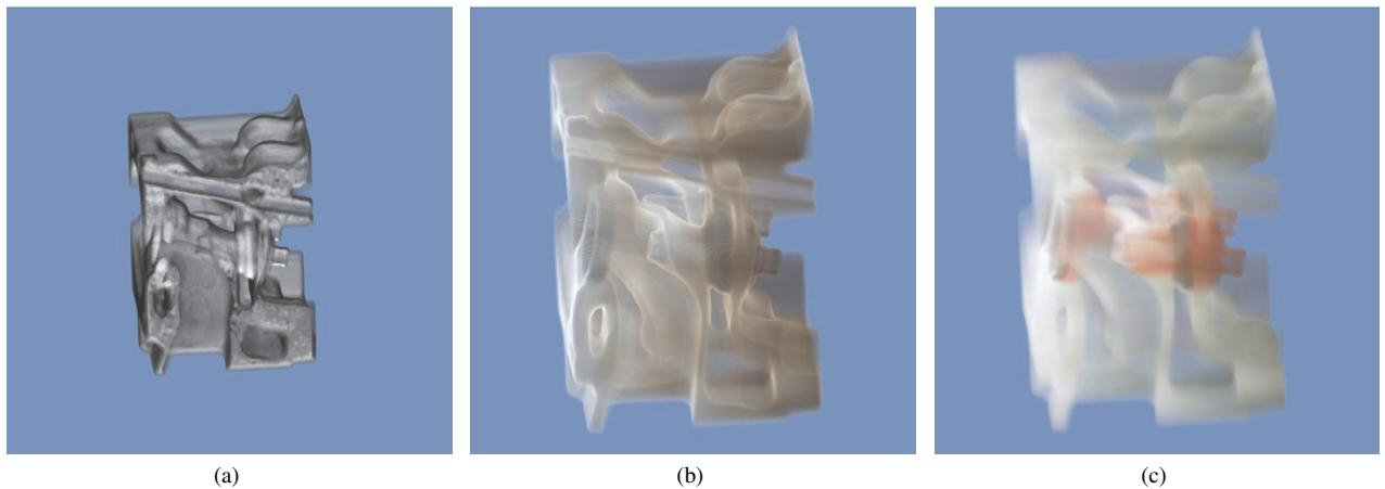
Fig. 7. Global illumination of an industrial CT scan of an engine. The original data is  $128 \times 128 \times 64$  and the sampled FCC lattice is  $136 \times 136 \times 98$ . The images are rendered with (a) ray casting with local illumination, (b) and (c) our multi-channel diffuse photon tracing.
