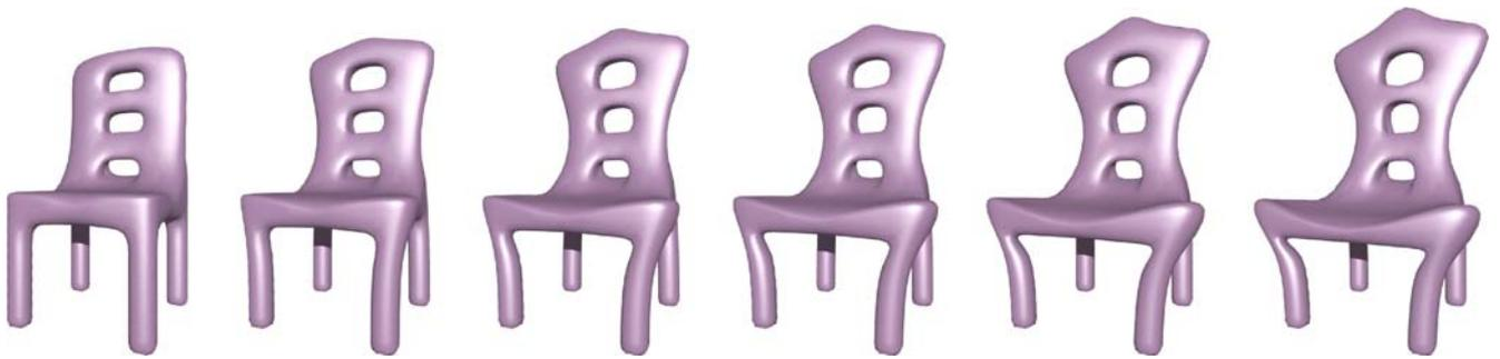
**Fig. 12.** A new chair is designed via force-based tools. Boundary constraints were imposed on the bottom portions of the legs to fix their positions
