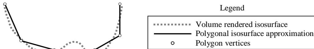
Figure 1: Polygonal isosurface approximation compared to volume rendered isosurface.
