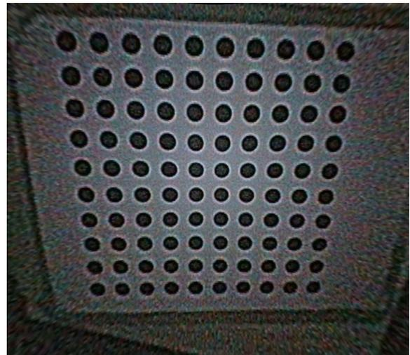
(f) Undistortion of image (b) with parameters  $k_1 = -0.027000$  and  $k_2 = 0.000175$ .
