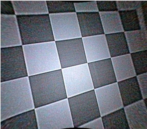
(c) Undistortion of image (a) with parameters  $k_1 = -0.024000$  and  $k_2 = 0.000000$ .
