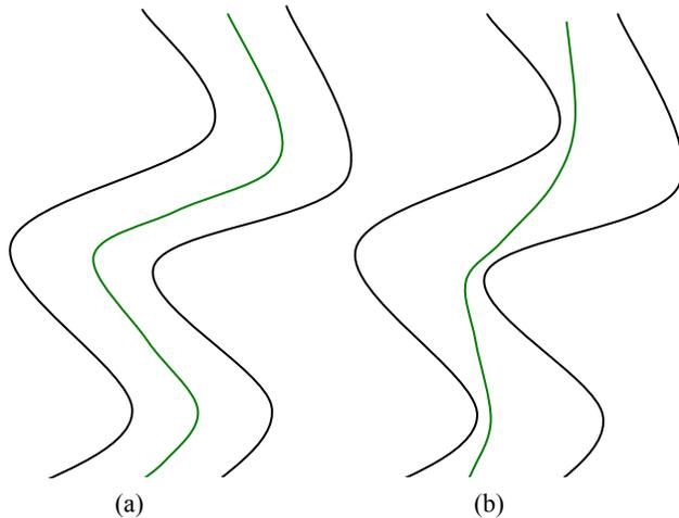
Figure 1: (a) An example of a centerline, and (b) a hugging corner shortest path.
