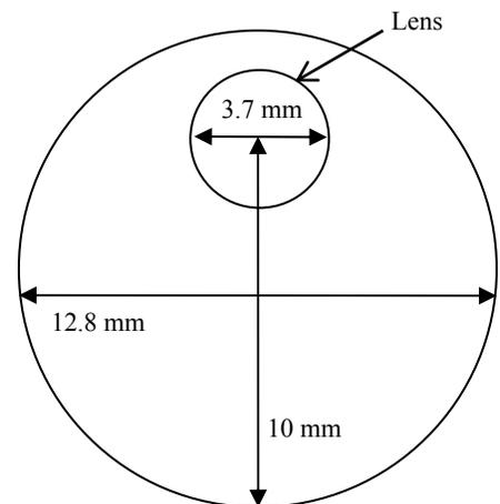
Figure 2: The location of the lens on the distal end of a colonoscope.
