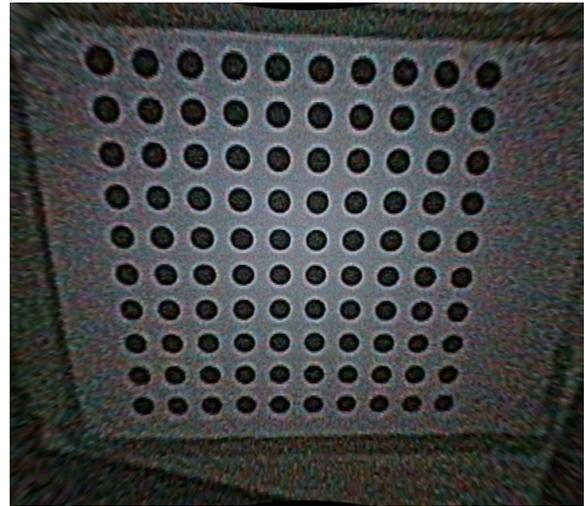
(d) Undistortion of image (b) with parameters  $k_1 = -0.024000$  and  $k_2 = 0.000000$ .
