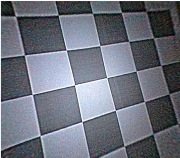
(e) Undistortion of image (a) with parameters  $k_1 = -0.027000$  and  $k_2 = 0.000150$ .
